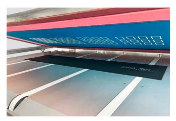
The card is held in place by means of a vacuum plate during the squeegee process. Accurate adjustment of stopping position.
