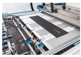
Automatic card-feeder with optical photo-cell monitoring of stack height.
