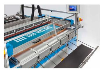
Automatic output of the glued card. Sensor-controlled triggering of the next gluing cycle.
